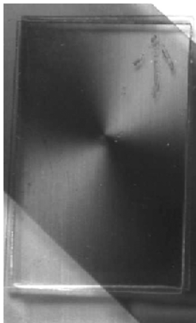
FIGURE 2 The circular NLC filter onto the polarizing sheet and seeing by means of the analyzer.
